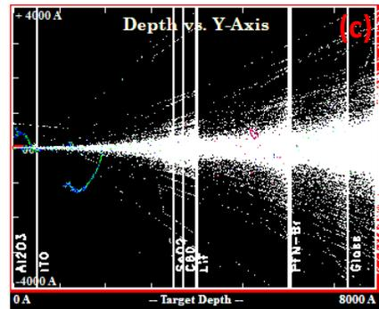
Trajectory of protons in the solar cell using SRIM
